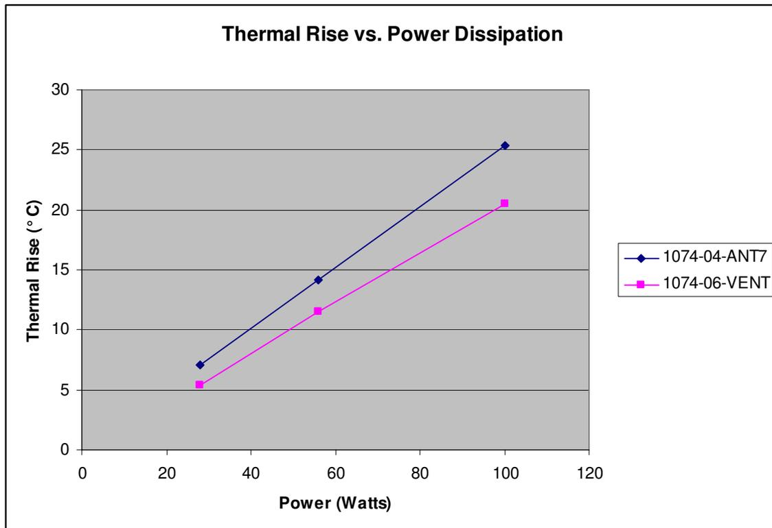
In the absence of measured power dissipation for the remote access unit, Oberon recommends de-rating the RAU manufacturer's operating temperature range by using the following equation based on the power dissipated, for the respective zone enclosures.
